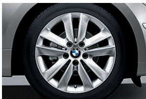
□ 17" light alloy wheels V-spoke 141 with runflat tyres, 7 J x 17, 205/50 R 17 tyres (standard on 123d).
