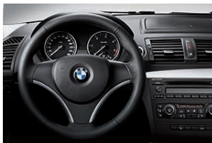
□ Sport leather steering wheel (diameter 369 mm) with thumbrests (in conjunction with gearshift paddles on the steering wheel without thumb rests), chrome clasp, three spokes (standard with 130i and 123d).
