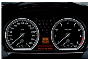
■ The instrument panel in the 130i features special scaling with an extended display and an oil temperature gauge.
