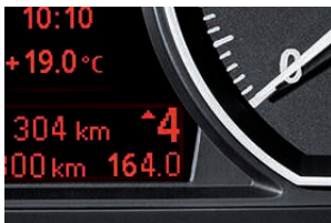
■ Optimum Shift Indicator shows when switching to another gear would be more fuel efficient. The system recommends when to switch to a higher or lower gear, as appropriate to your driving style. For example, when you accelerate it signals whether to carry on accelerating in a higher gear, thereby saving fuel (for vehicles with six-speed manual transmission).
