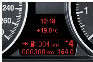
■ On-board computer , provides information about average speed, average and current fuel consumption, range and outside temperature. It also features an acoustic ice warning.
