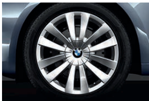
□ 20" light alloy wheels Double-spoke 253 with mixed tyres, front 8.5 J x 20 with 245/40 R 20 Y tyres, rear 10 J x 20 with 275/35 R 20 Y tyres.
