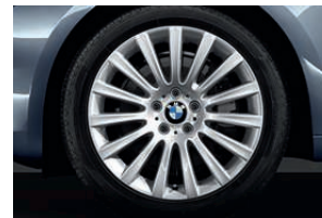
□ 19" light alloy wheels Multi-spoke 235 with mixed tyres, front 8.5 J x 19 with 245/45 R 19 Y tyres, rear 9.5 J x 19 with 275/40 R 19 Y tyres.
