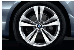
□ 20" light alloy wheels Double-spoke 316 with mixed tyres, front 8.5 J x 20 with 245/40 R 20 Y tyres, rear 10 J x 20 with 275/35 R 20 Y tyres.
