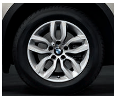
□ 17" light alloy wheels Y-spoke 305 , 7.5 J x 17 with 225/60 R 17 tyres, also available as a complete winter wheel set from the Original BMW Accessories range*.
