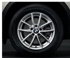
■ 17" light alloy wheels V-spoke 304 , 7.5 J x 17 with 225/60 R 17 tyres (standard with X3 xDrive20i and X3 xDrive20d), also available as a complete winter wheel set from the Original BMW Accessories range*.
