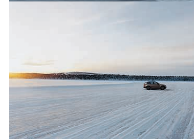
The low frictional coefficients on the frozen lakes are perfect for repeatable test drives out at the limits.
