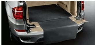
Luggage compartment reversible mat can be used either way up, and is non-slip.
