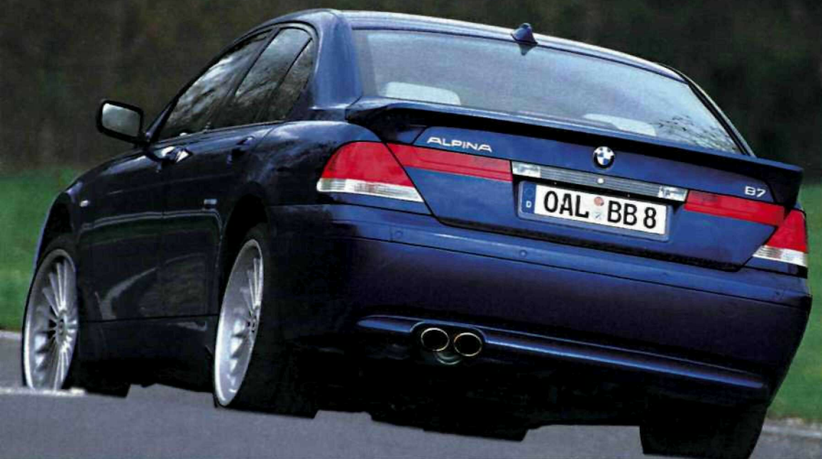
FORM AND FUNCTION The air duct at the rear suits the 7-series particularly well and reduces lift
