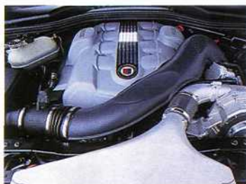
V8 produces 516lb ft of torque: 173lb ft more than the M5's V10; bespoke trim makes it feel more special
