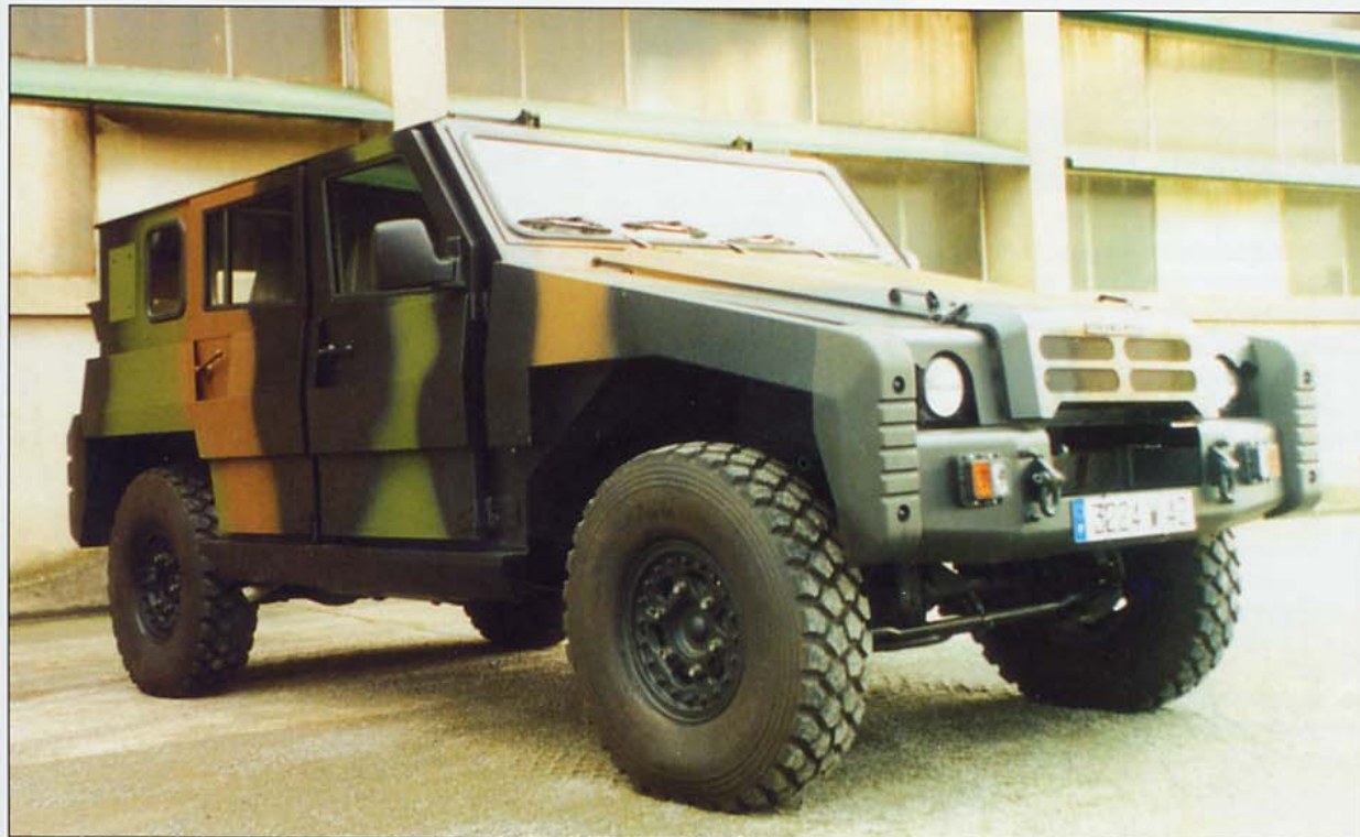
Top left; some years ago Auverland developed an armoured variant of the A3 as a private venture, the type remains available.
