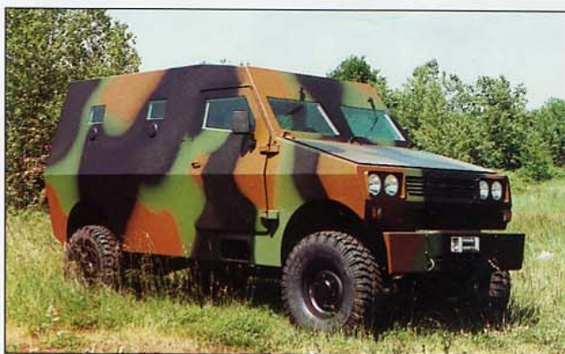
Top left; some years ago Auverland developed an armoured variant of the A3 as a private venture, the type remains available.
